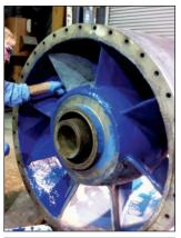
CeramAlloy CL+AC used to coat all surfaces.
