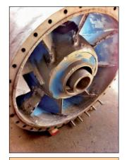
The severely eroded vanes were cut away.
