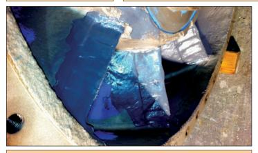
CeramAlloy CP+AC used to rebuild the vanes to their original size.
