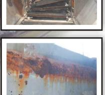
The largest coal-fired power plant in the Philippines (1300 MW generating capacity) had a serious corrosion cost effective solution problem on their two Submerged Scraper Conveyors (SSC). These mechanical drag paint systems that had conveyors help remove bottom ash from below the boiler units.
